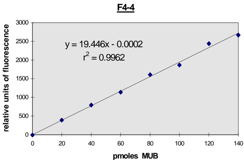
Figure 3-2: example of a AMC calibration curve (sample F4-4)
